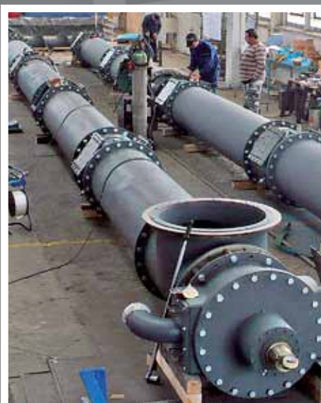
Assembly of vertical conveyors
