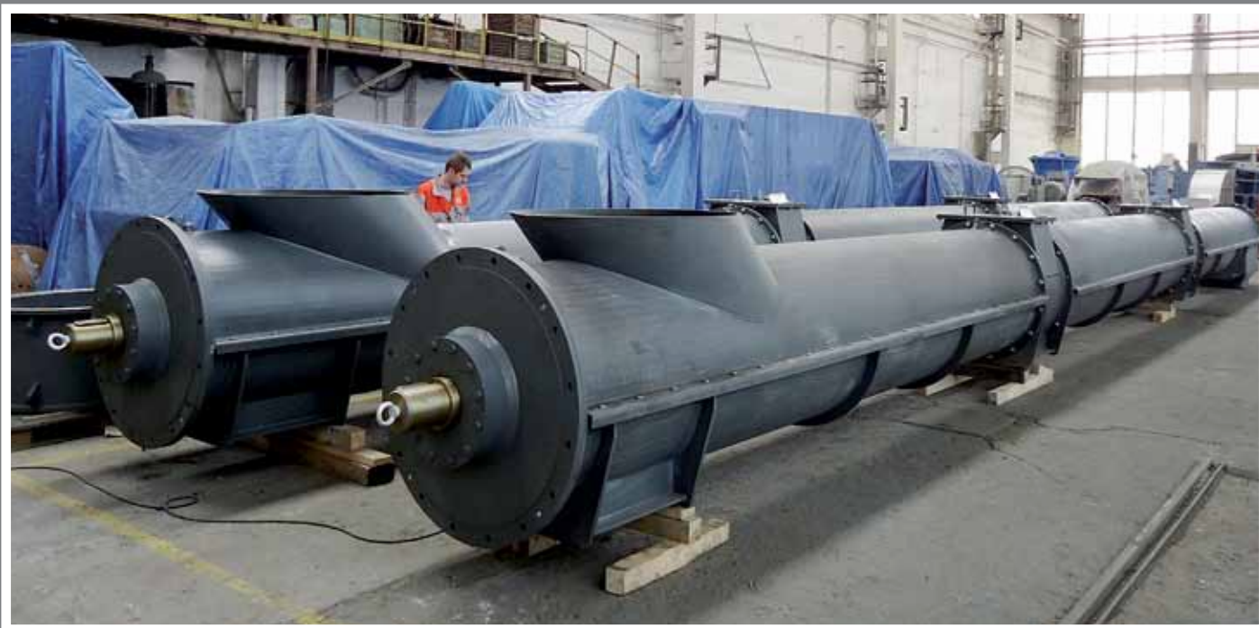
Assembly of horizontal conveyors
