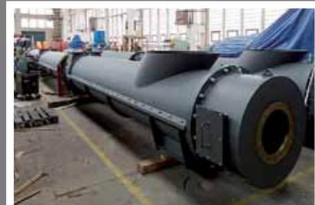
Assembly of horizontal conveyors
